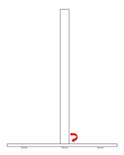
1.4. After you have securely screwed the stand to the base plate, you can now insert the heating head into the telescopic holder from above. Make sure that the opening hole for the locking Allen screw is (becomes) visible through the counter opening of the heating head! Now tighten (close) the lock for the telescope height.
